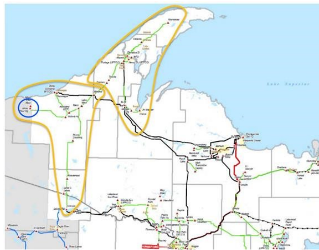
Map shows ATC's transmission system in the western Upper Peninsula. The orange circles indicate how the load pocket will be split into two radially fed areas. Location of White Pine Unit 1 circled in blue on upper left of map. Source: MISO
